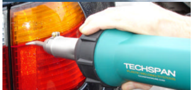
Tacking prior to welding
