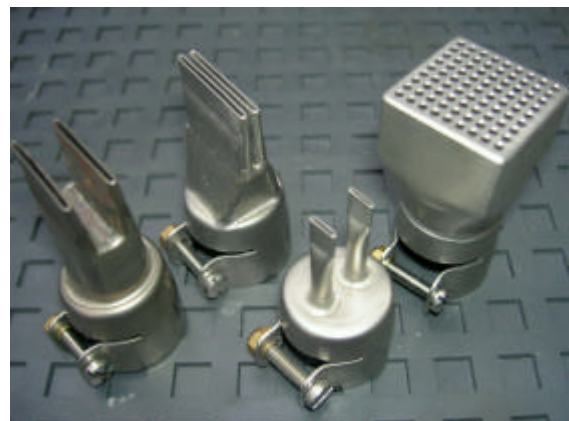
Selection of soldering/desoldering nozzles for the HotJet S tool
