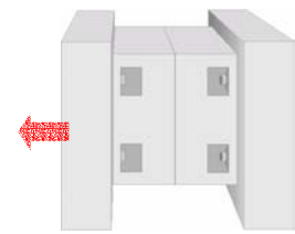
Figure 4.7 Remove crane, mould can be opened
