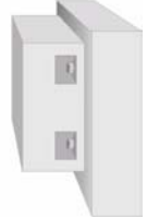
Figure 4.3 Apply moving mould half with crane balance centrally on moving mould fixing platen
