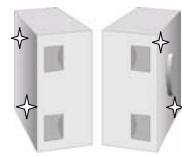
Figure 4.1 Pull off mould fixing platens and mould outer surfaces with oil rubber, clean grease-free
